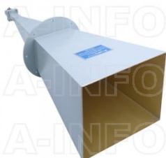
LB-90-25-C2-3.5F Standard Gain Horn Antenna 8.2-12.4GHz 25dB Gain 3.5mm Female
